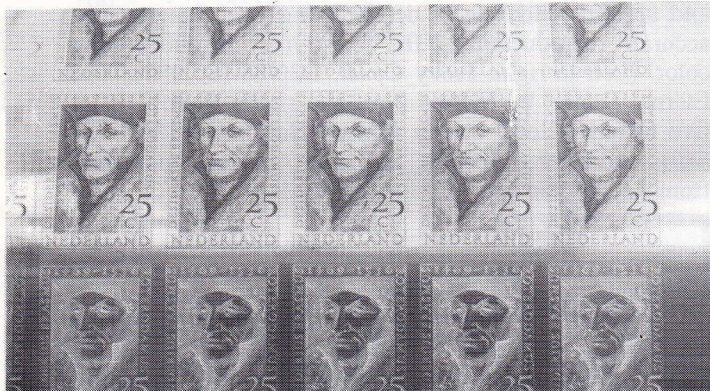
A recess printing plate, partially inked
